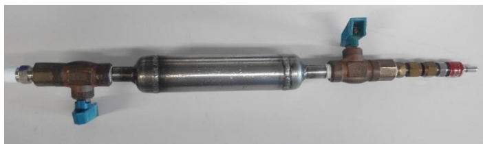
Figure 23 - Cartridge used to inject the iso-hexane in the reactor.
