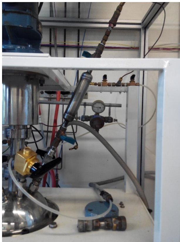
Figure 24 - Cartridge with iso-hexane linked to the reactor.
