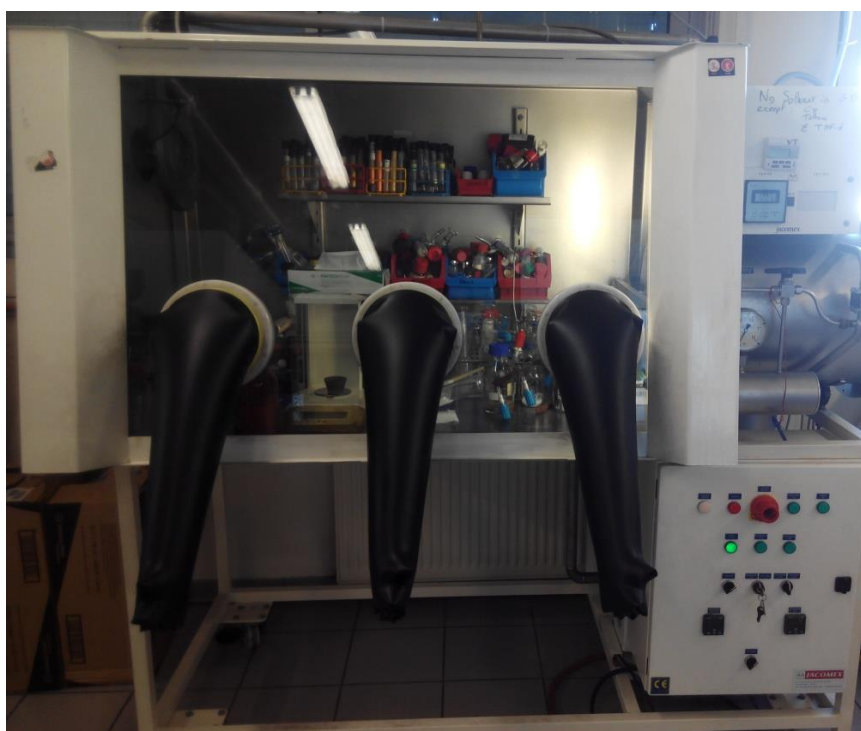
Figure 20 – Glovebox used for precatalyst and alkane preparation.
