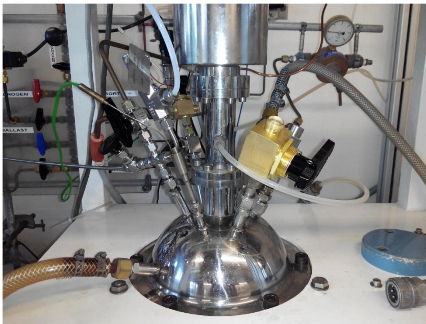
Figure 19 - Reactor used for propylene polymerization.
