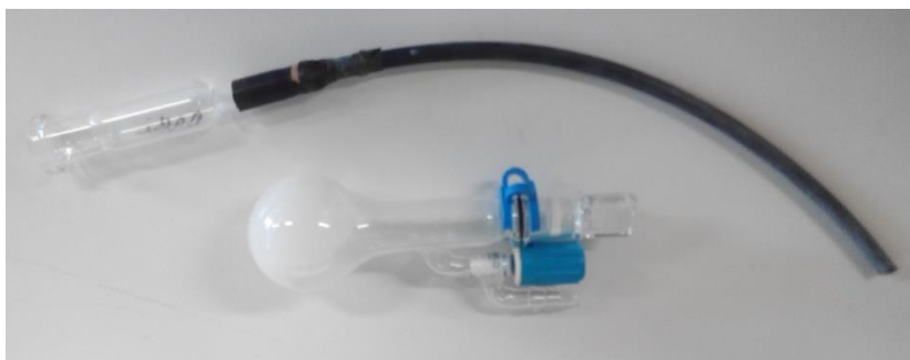
Figure 21 - Schlenk with mixture of catalyst and salt and cup with hose for injection in the reactor.
