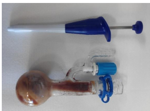
Figure 22 - Schlenk with mixture of oil and catalyst and micro-pipette for its injection.
